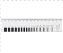
CW01 Crack Width Gauge
