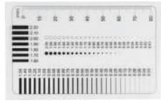
CW02 Crack Width Ruler
