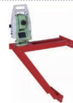
IWB02 Instrument Wall Bracket • A Solid Designed Wall Bracket made from 50mm Angled Steel • A Square 200 x 200 x 10mm Plate is Supplied with a Fixed (non-rotatable) 5/8" screw • Mounting is Carried Out using Four Heavy Duty M10 Anchor Bolts • Four Plating Pieces are Welded on the Back Side of the Wall Attachments to Guarantee Highly Reliable Positioning, Three Distances from the Wall are Available
