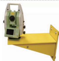
IWB01 Steel Instrument Wall Bracket • A Solidly Designed Monitoring System of Steel Wall Plates and Demountable Tables for Surveying within Tunnels • Centring is Better than 0.25mm. • Back Plate: 10kg, 380 x 254 x 10mm. Table: 9kg, 535 x 254 x 10mm
