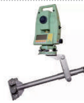
IWB04 Stainless Steel Instrument Wall Bracket • The Assembly and Horizontal Adjustment is Done in Less than a Minute • The Clamping Mechanism Allows Use of Even the Heaviest of Instruments with a Load in Excess of 80kg • A Rotatable and Tilttable Hinged Arm and Instrument Plate Means the Instruments Can be Fixed into Almost Every Position • Length: 540mm
