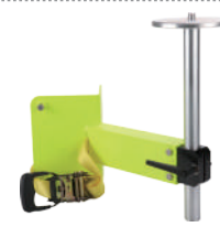
HDCC01 Heavy-Duty Column Clamp • The Adjustable Column Rotates and Moves Vertically to Orient the Instrument • Use for All 5/8"-11 Instrument • Heavy Duty Ratchet to Create a Strong Connection to Both Round and Square Columns
